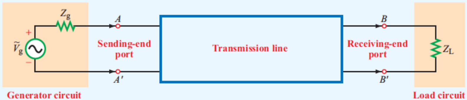
Figure 2-1 A transmission line is a two-port network connecting a generator circuit at the sending end to a load at the receiving end.
