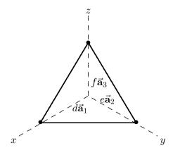
Let  $\{def\}$  be the smallest intercepts as multiples of the three lattice parameters representing a given set of planes. The inverses of these are  $\{1/d, 1/e, 1/f\}$ . Multiplying this by m, the LCM of  $\{def\}$ , gives the Miller indices:
