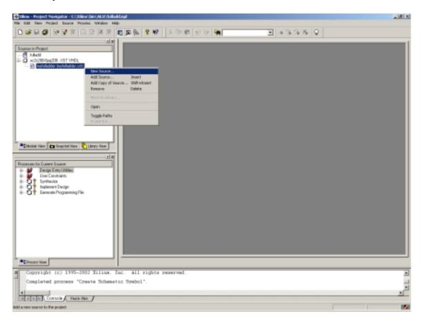
This will open a dialog box, prompting you to enter a choice for the design type and a name. Select "Test Bench Waveform" as the type of design entry. Also make sure you don't forget to name your file.
