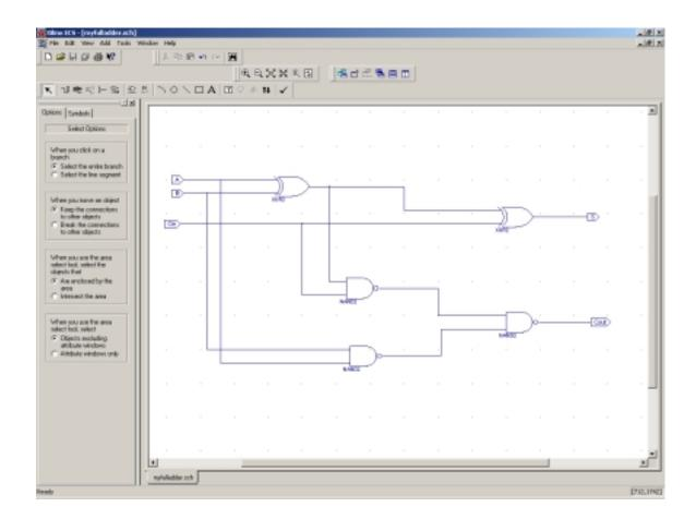
The full adder as three inputs (A, B, Cin) and two outputs (S, Cout). Now save your schematic and close the Schematic Editor.
