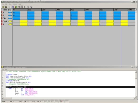
Various values (0 or 1) can be assigned to the inputs by just clicking on the blue bar corresponding to each input.
