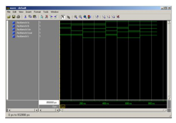
Take a look at the Wave window. In this window we are able to see the waveforms of our design that we just simulated, the full adder.
