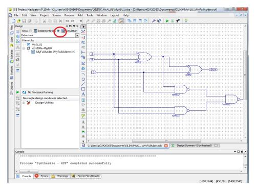
3. Next, go back to the Project Navigator. Highlight the source that you want to simulate. In this case, we want to simulate the circuit named MyFullAdder. Then, right click on the source MyFullAdder and select New Source.
