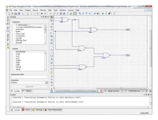
The full adder has three inputs (A, B, Cin) and two outputs (S, Cout). If you have not yet saved your schematic, do so and close the Schematic Editor.
