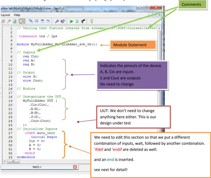
And under the **Initialize Input**, we need to assign different test cases. Since, we have three inputs A, B, and C, they could take on values from 000 to 111. For each case, we put the value for A, B, and C and then wait for a few nanoseconds before repeating the process for a different input combination.
