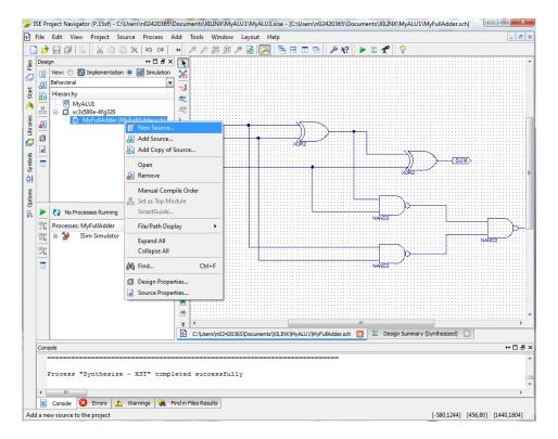
4. This will open a dialog box. Select "**Verilog Test Fixture**" as the type of design entry and pick a name for your test-bench file.
