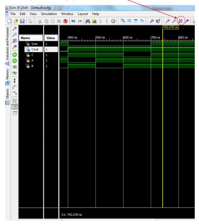
You can position the cursor on the various points and see the corresponding value displayed on the left side of the display. For example, for the current cursor position, C=1, A=1, B=1 resulting in Sum=1 and Cout=1; which is the correct result.
