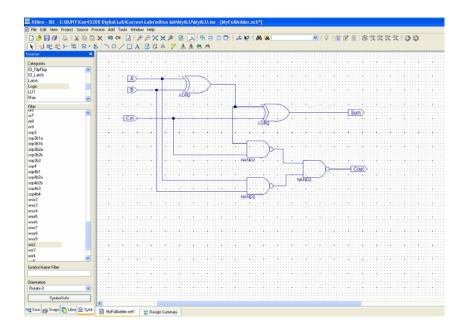
The full adder has three inputs (A, B, Cin) and two outputs (S, Cout). If you have not yet saved your schematic yet, do so and close the Schematic Editor.
