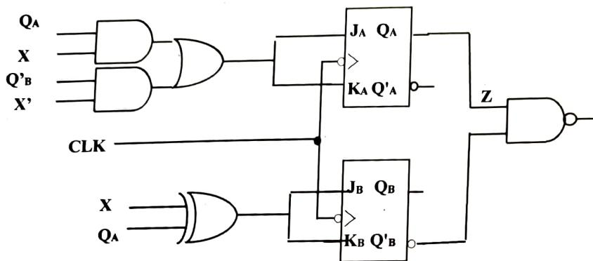
$$1. \quad J_A = K_A = Q_A X + \bar{Q}_B \bar{X}$$
