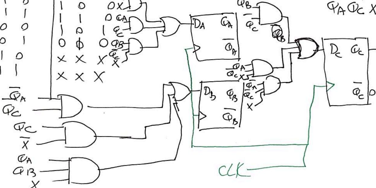
Analyze the following circuit leading to its state diagram.
