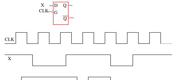
Problem 3 Complete the timing diagram if the following signals are applied as indicated.
