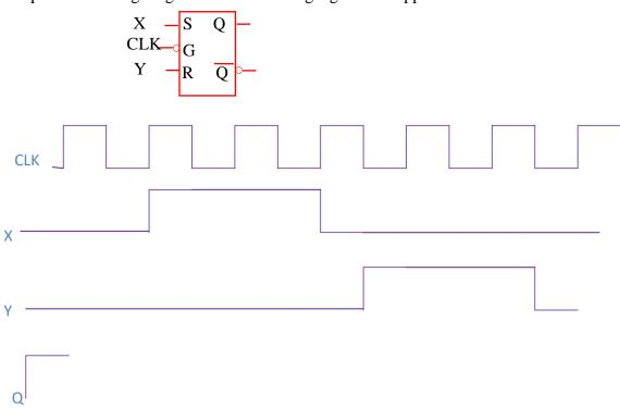
Problem 4 Complete the timing diagram if the following signals are applied as indicated.
