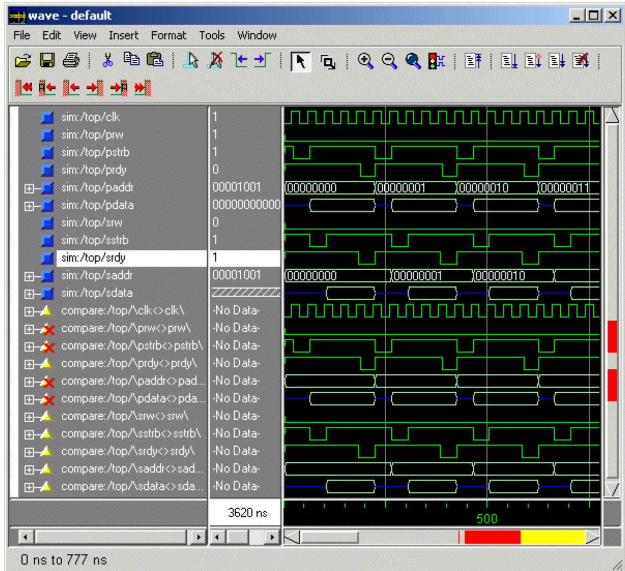
The Compare tab in the Main window shows the region that was compared, and the transcript area shows the number of differences found between the timing of the Reference and Test datasets.
