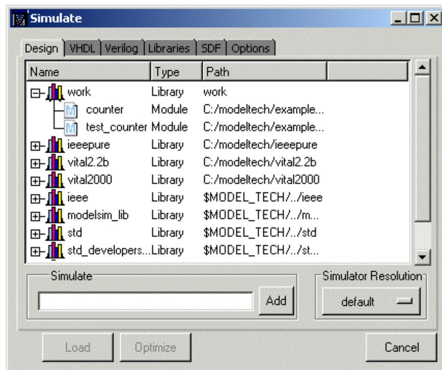
The Simulate dialog allows you to select a design unit to load from the specified library. You can also select the resolution limit for the simulation. The default resolution is 1 ns.
