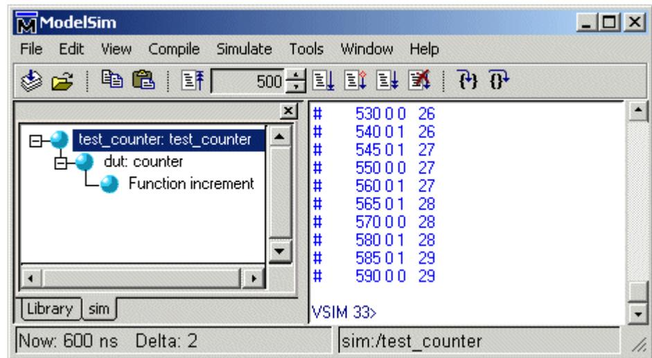
Now the simulation has run for a total of 600ns (the default 100ns plus the 500 you just asked for). The status bar at the bottom of the Main window displays this information.
