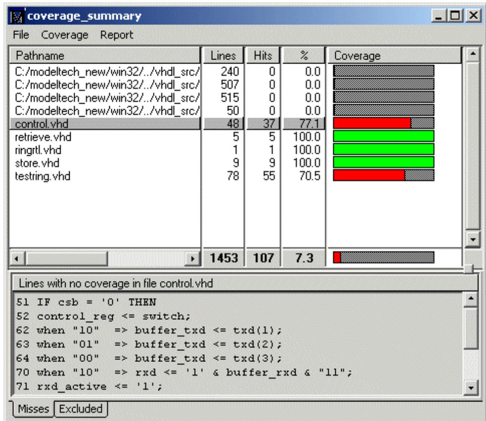
The top half of the window shows summary information on a per-file basis. If you select a file in the list, the bottom part of the window gives details about the lines in the file that have zero coverage.
