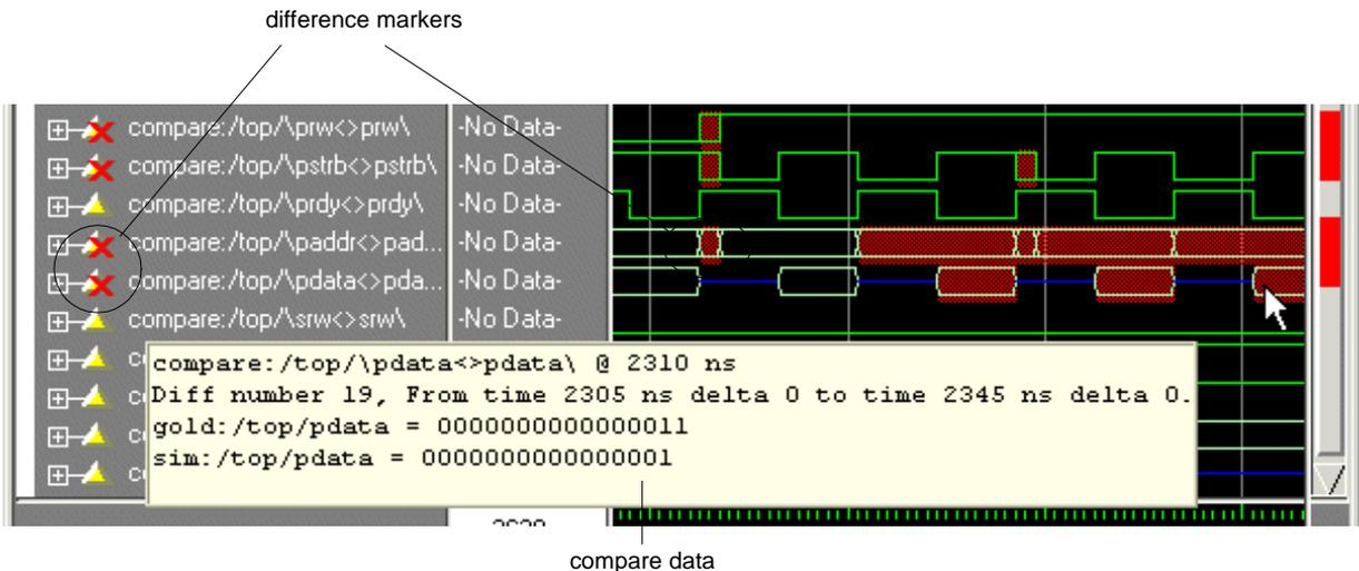
Hover your mouse pointer over a difference marker to display a popup containing data about that timing difference. Also note that when you place a waveform cursor over a difference, the values column displays the text "diff."
