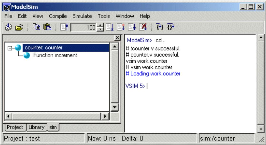
At this point, you would generally run the simulation and analyze or debug your design. We'll do just that in the upcoming lessons. For now, let's wrap up by ending the simulation and closing the project. Select **Simulate > End Simulation** and confirm
