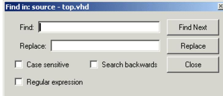
In the **Find:** field, type `cache_set` and click **Find Next**. The `cache_set` instantiations are now displayed in the Source window. (Click **Close** to dismiss the **Find in:** dialog box.)
