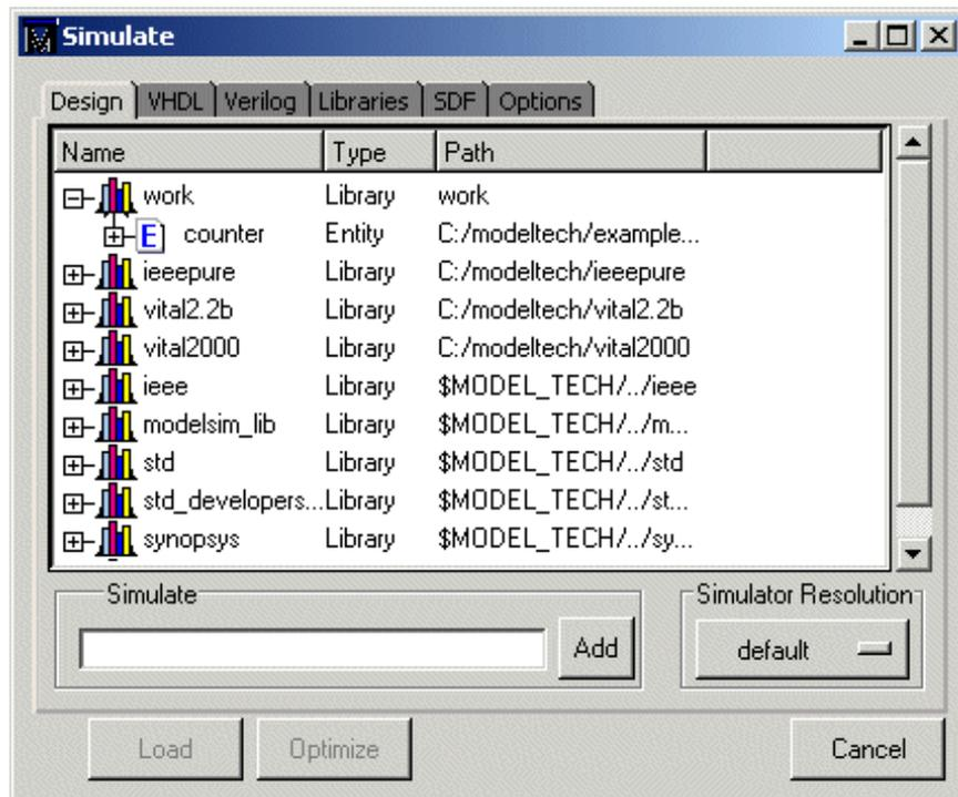
If the Design Unit is an entity (like **counter** in this design), you can expand it to view any associated architectures.
