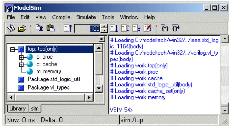
Notice the hierarchical mixture of VHDL and Verilog in the design. VHDL levels are indicated by a square “prefix”, while Verilog levels are indicated by a circle “prefix.” Try expanding (+) and contracting (-) the structure layers. You’ll find Verilog modules that have been instantiated by VHDL architectures, and similar instantiations of VHDL items by Verilog.
