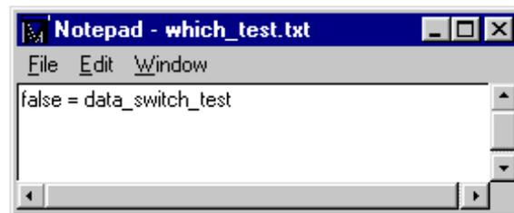
This switch configures the test bench – the `ringrtl.vhd` file. We'll change it later in the lesson when we merge the coverage results of two simulations.
