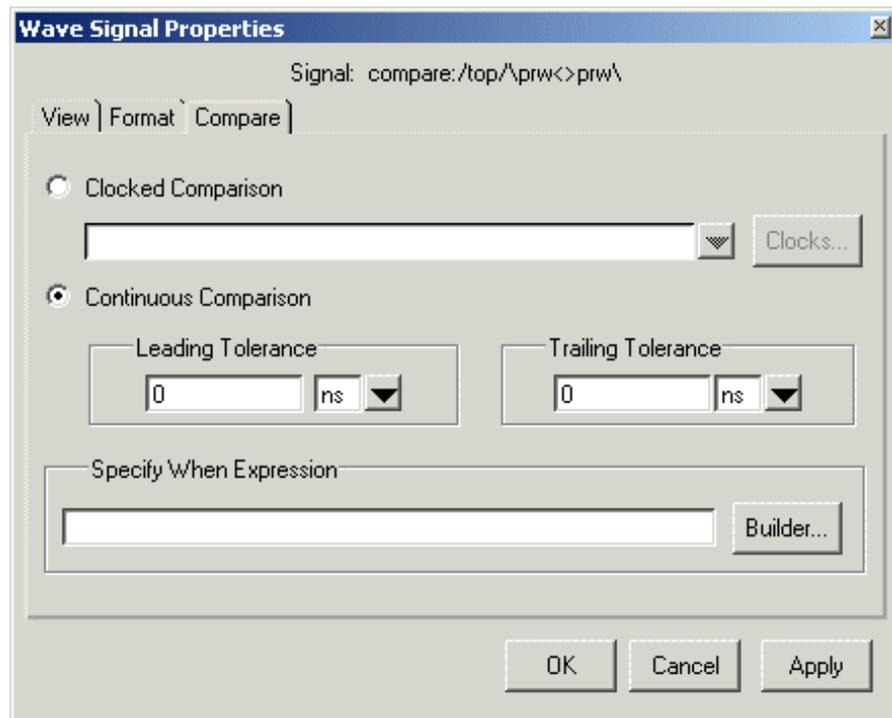
Recall that we delayed the read cycle in *proc.v* by 10 time units. Therefore, if we specify a trailing tolerance of 10 ns, the differences on the comparison object should disappear.
