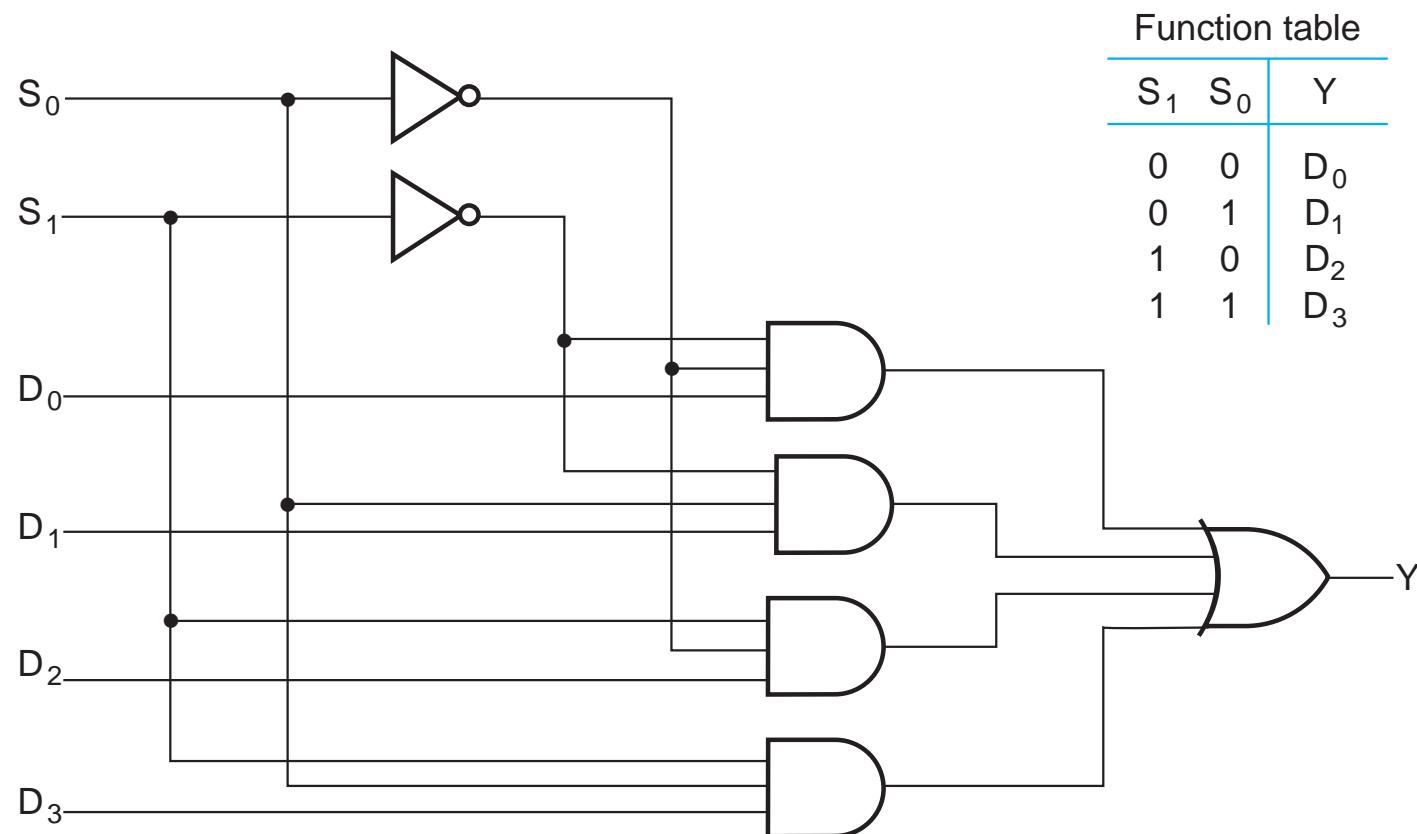
**Figure 3-37 Structural VHDL Description of a 4-to-1 Line Multiplexer**
