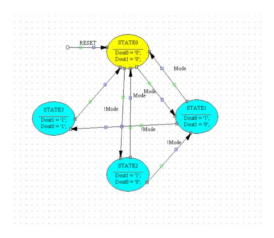
For multiple inputs, you can either Abel notation A & !B & C or using VHDL notation A='1' AND B='0' AND C='1'.
