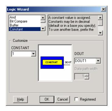
Do this process again. But, this time, define an output "DOUT2" with data width 1 and set its constant value to 0. Click "OK". Now State 1 has two defined outputs.
