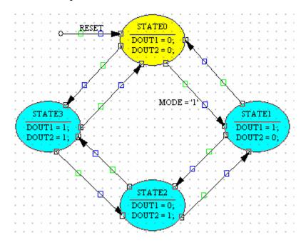
If a state transition is not needed, it can be deleted by left clicking on the transition line and pressing the delete key. Let's delete the following state transitions.
