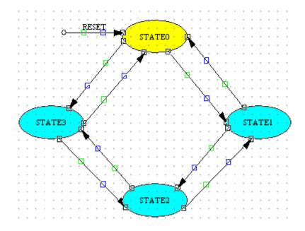
Now that the basic diagram is in place, we need to add/remove/modify the current transitions to obtain the correct state diagram for the sequence generator. Left-click on one of the two boxes of the transition arrow **State0-->State1**. This will bring up the "Edit Conditions" dialog box. Add the condition **MODE = '1'** in the "Conditions" box.
