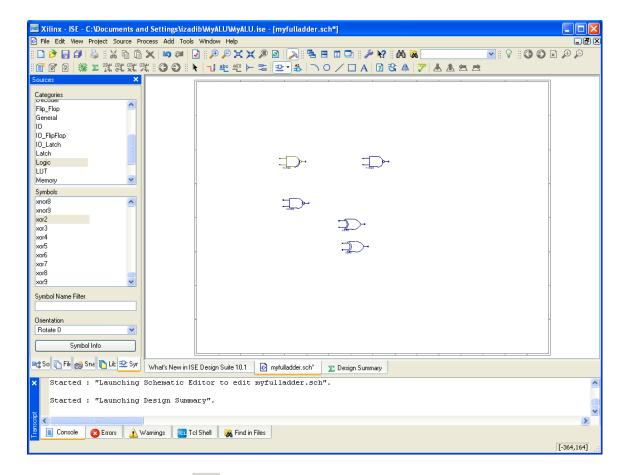
2. Click on the Add Wire icon. This will allow you to connect the components together. Click on the lead of one gate then on the lead of the next and a wire will be drawn that connects the two together. Note that
