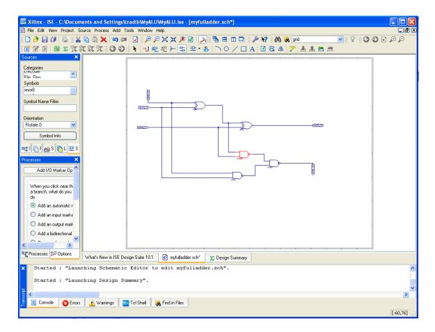
Your schematic should look like this with the markers in place. Xilinx automatically assigns names to the markers, but remembering the names can get confusing really fast.
