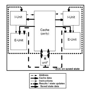
Fig. 3. Logical layout of the zSeries microprocessor chip.
