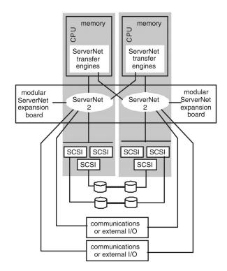
Fig. 5. Tandem NonStop Server S-series architecture (two processors shown).
