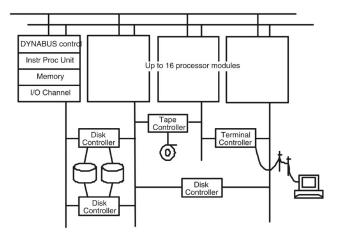
Fig. 2. Original tandem system architecture (1976).
