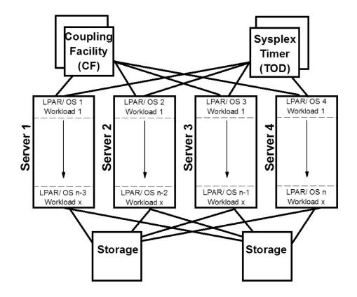
Fig. 4. zSeries parallel sysplex architecture.
