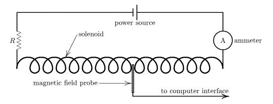
The above setup is used to make the measurements. **Do not let the current rise above 2.0 A.** The computer continuously monitors the magnetic field measured by the probe. The direction of the field measured is marked on the probe. For a given orientation of the probe, its measurement must be zeroed with the current set at zero. This makes sure other sources of magnetic field (in particular the Earth) do not interfere.
