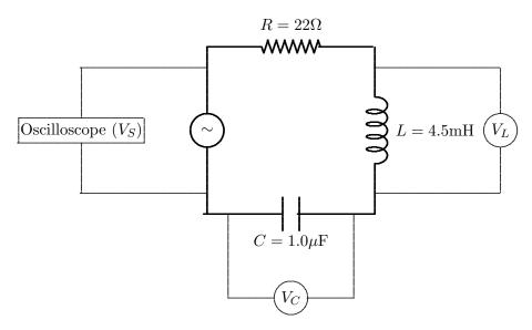
A series RLC circuit with AC input is shown above. A voltmeter is connected across the inductor to measure the rms voltage  $V_L$  across it. Similarly, another voltmeter measures the rms voltage  $V_C$  across the capacitor. An oscilloscope is connected across the source function generator to observe the waveform as well as measure the rms voltage  $V_S$  delivered. A sinusoidal input voltage from the source is written as follows.
