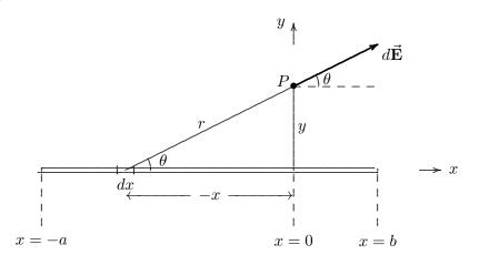
In the figure above the origin of a xy coordinate system is chosen on the rod a distance a from its left end. The rod is along the x axis and the point P is on the y axis. For  $E_x$ , the x component of the electric field, we see that an element of rod of length dx produces the field
