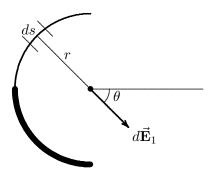
For the top quarter circle, the charge density is  $\lambda_1 = 2q/(\pi r)$ . The electric field due to the element ds is  $d\vec{\mathbf{E}}_1$ . The x and y components of this field are:
