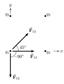
The force on charge  $q_1$  due to  $q_2$  is  $\vec{\mathbf{F}}_{12}$ . From Coulomb's law, the magnitude of this force is,
