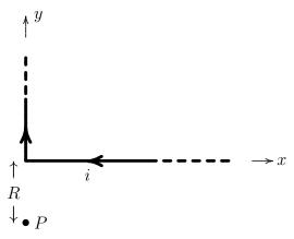
A long thin wire is bent in the shape shown above. Assume it extends to infinity in the positive y and positive x directions as shown. A current i flows in the wire as shown. The point marked P is at a distance R along the negative y axis as shown.
