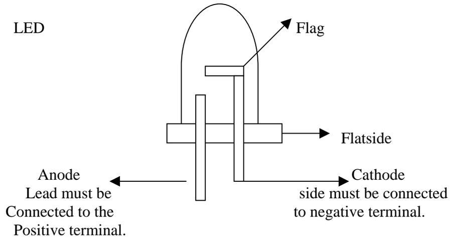
The light-emitting diode is a solid state device that will light when it is forward-biased by approximately more than 2v when it starts to emit a visible light. The light can be red, green, orange, white or blue depending on the chemical structure of the material. Forward biasing the diode means connecting the anode to the positive terminal of the source and the cathode to the negative side of the source.
