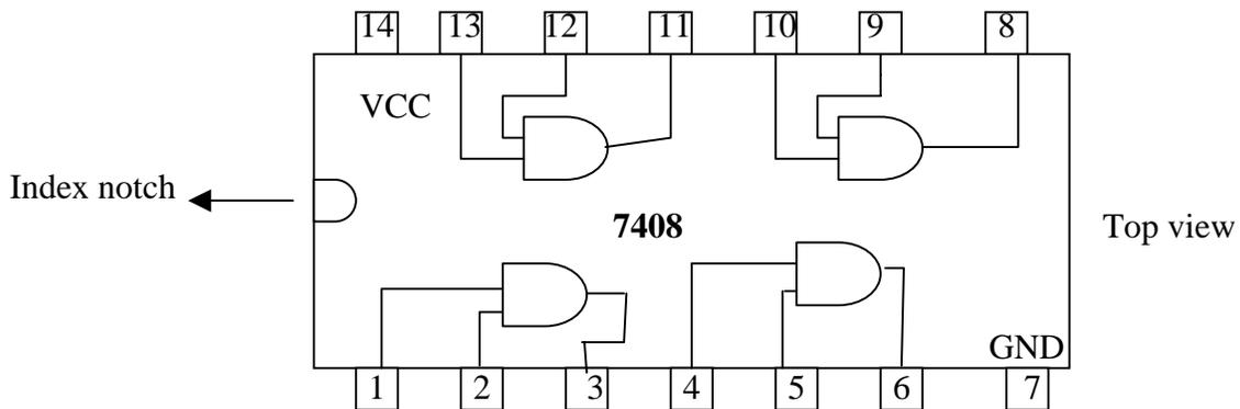
The above pinout is that of a 7408 quad two-input AND gate which has a 14 pin configuration and a TO-116 EIA packaging designation.
