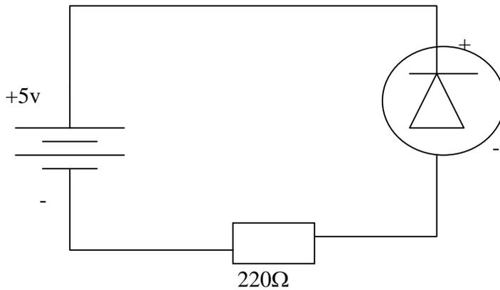
LED is reversed biased and will behave as an open switch. No current will flow and it will not emit light. The advantage of an LED over an incandescent light bulb is low power consumption and longer life.
