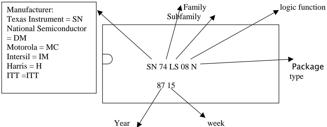
54HC / 74HC means a CMOS chip that is pin for pin compatible with TTL 54LS/74LS.
