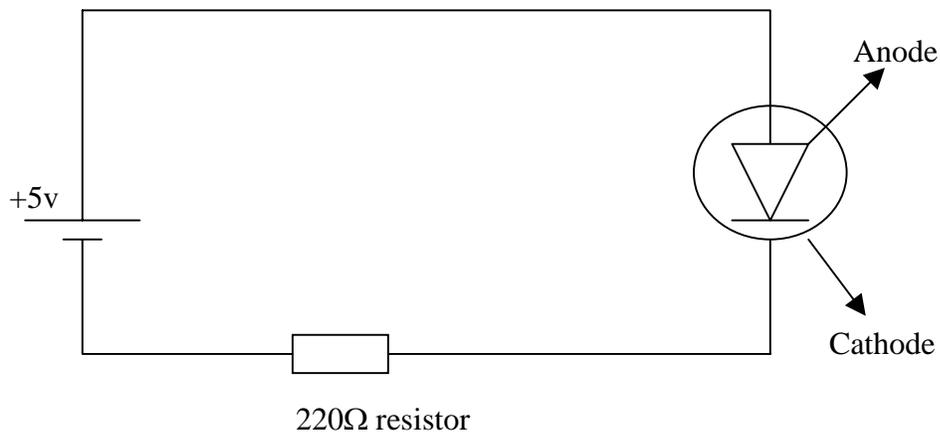
Always use a series resistor with an LED. LED is forward biased by more than 2v. It will emit light and current will flow.
